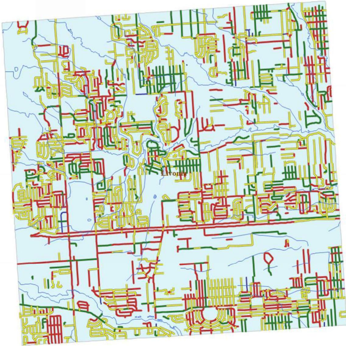
Figure 7: Map showing location of City of Livonia DPW's paved roads (i.e., those managed by City of Livonia DPW) and their current condition for paved roads with green for good (i.e., PASER 10, 9, 8), yellow for fair (i.e., PASER 7, 6, 5), and red for poor (i.e., PASER 4, 3, 2, 1), as well as the location of City of Livonia DPW's unpaved roads in blue.
