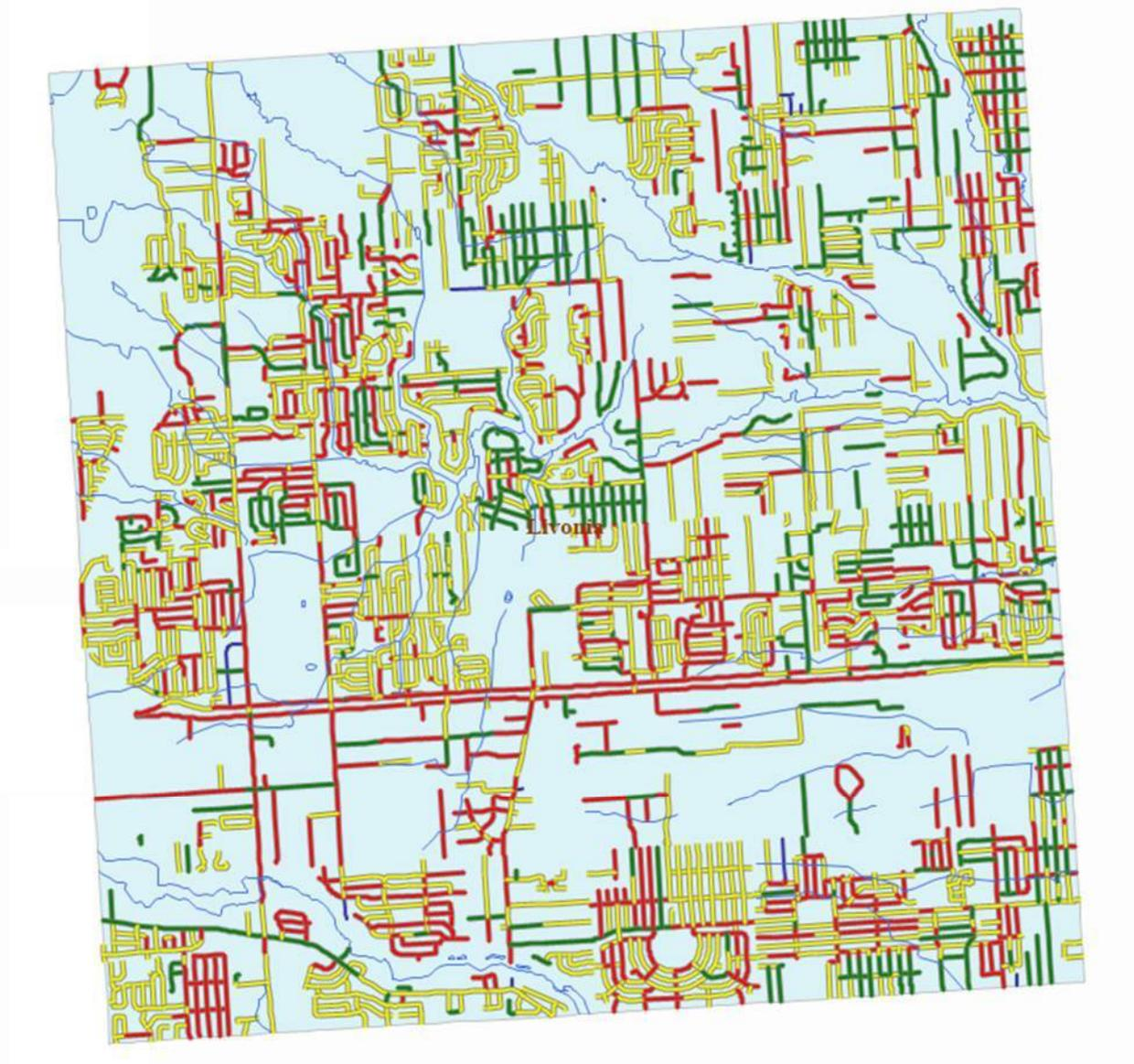
Figure 1: Map showing location of roads managed by City of Livonia and the current condition for paved roads in green for good (PASER 10, 9, 8), yellow for fair (PASER 7, 6, 5), and red for poor (PASER 4, 3, 2, 1) and for unpaved roads in blue from 2023.
